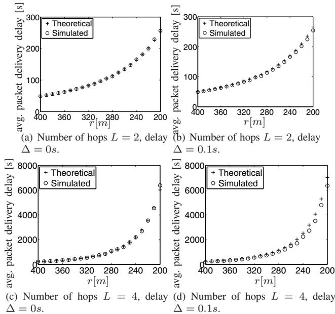
Fig. 3: Comparison of theoretical and simulated curves of the IP-like average packet delivery delays for different values of transmission radius  $r$ , number  $L$  of hops, and  $\Delta$ .
