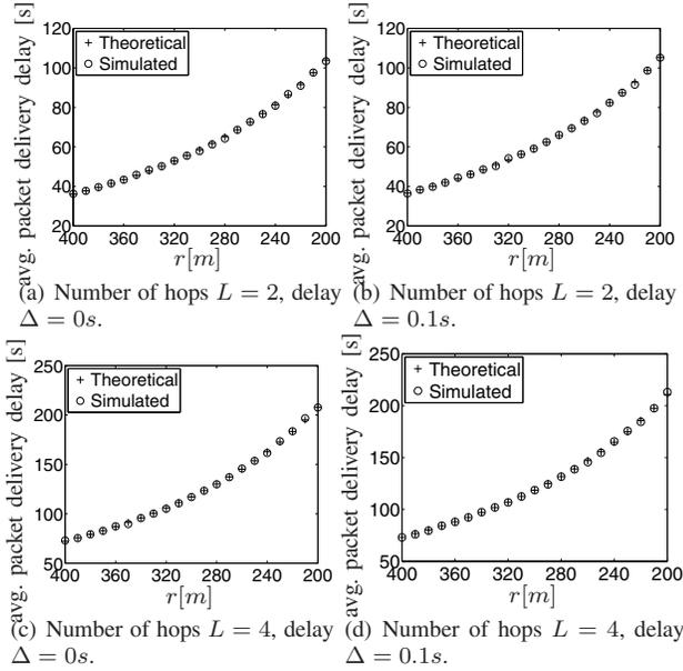
Fig. 2: Comparison of theoretical and simulated curves of the DTN average packet delivery delays for different values of transmission radius  $r$ , number  $L$  of hops, and  $\Delta$ .
