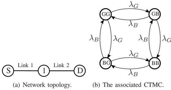
Fig. 1: A simple two-hop network topology (a) and the associated CTMC, whose nodes represent the sets of configurations of its links (b). The parameters  $\lambda_B$  and  $\lambda_G$  are the non-zero transition rates between different states of the CTMC.
