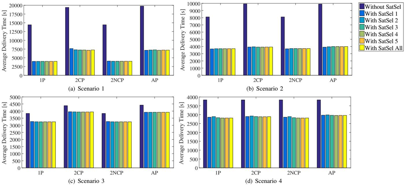
Figure 4: Average delivery times bursty bundles traffic flow configuration
